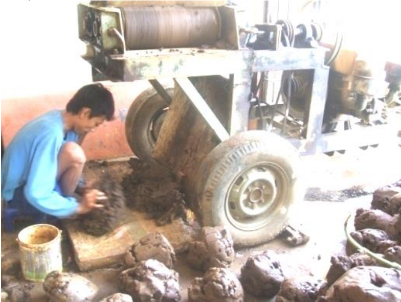
Fig. 2 Processing clay ceramic materials with a double cylinder rotating machine
